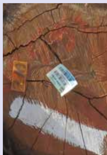
Barcode on log from PNG. The code relates to a specific logger and license area.
