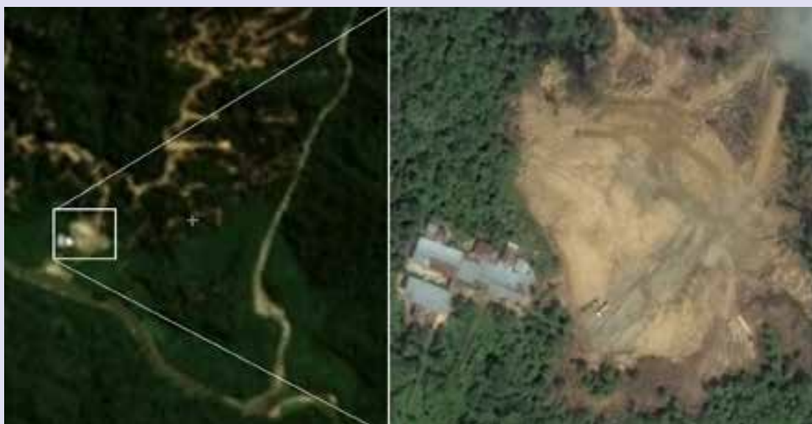
Left: 15m-resolution Landsat 8 image showing fresh roadbuilding and intensive selective logging. Right: 50cm-resolution Worldview 2 image of part of the same area, with buildings, vehicles and individual logs visible.
