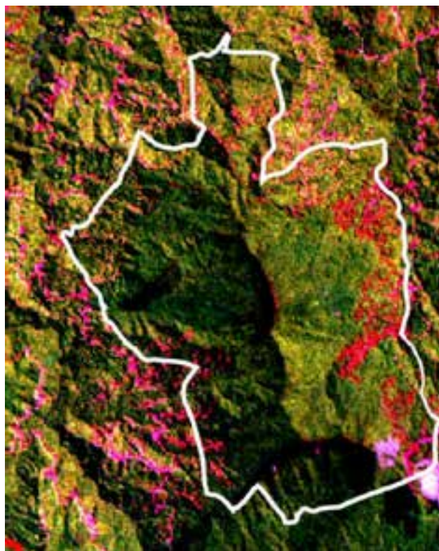
Landsat image with vegetation damage highlighted using false colouration of infra-red bands. Logging roads show up pink; recent intensive logging activity in red, areas logged earlier in light green. This technique can identify recent selective logging activity. This image shows logging inside the protected Batu Lawi mountain area in Sarawak by Malaysian company Samling. ©EarthSight
