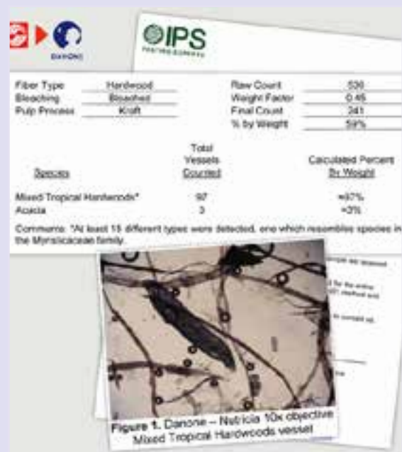
Greenpeace has commissioned fibre analysis to identify tropical hardwoods in paper samples. Photo reproduced with permission of Greenpeace and IPS Inc.
